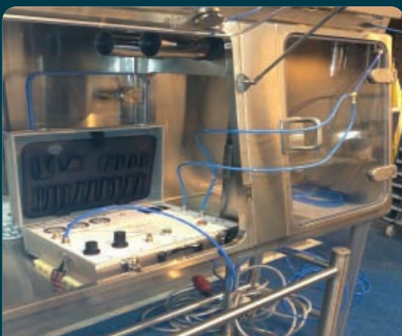
The Valiflate - can be used at a clients premises to validate seal performance and durability
